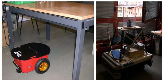
Fig. 1. Robots without 3D perception cannot clean under the table (left) neither avoid bumping into the open window (right).
