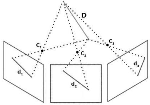
Fig. 3. 3D segment-based reconstruction for a trinocular stereoscopic system.
