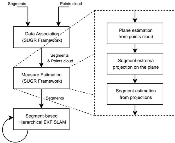
Fig. 4. The sensor fusion mechanism
