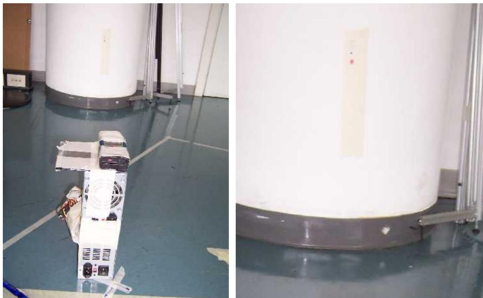
*Picture showing how the actual measurements of the robot-frame point to the world-point were taken. Notice that only the horizontal (and not the vertical) alignment is reached.*
