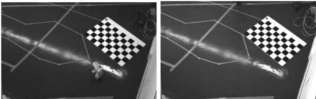
Images used to evaluate the error between the estimates of a chessboard in the same pose, before (left) and after (right) the data collection.
