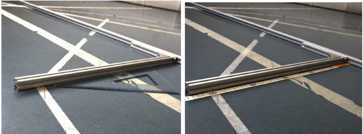
Pictures showing how the initial guesses based on the mechanical frame were taken; other initial guesses were taken by "eye determination" of the intersection, with the x axis, of a line parallel to the y axis and passing through the origin of the robot-frame; such intersection determined, along the x axis, the x coordinate of the origin of the robot-frame, while the length along the line was the y coordinate; the orientation was also the result of "eye determination".
