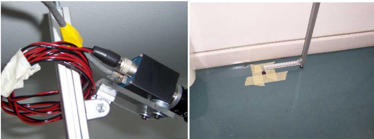
*A camera connected from behind (left) and pieces of paper-tape around the pole to detect undesired rotations (right).*
