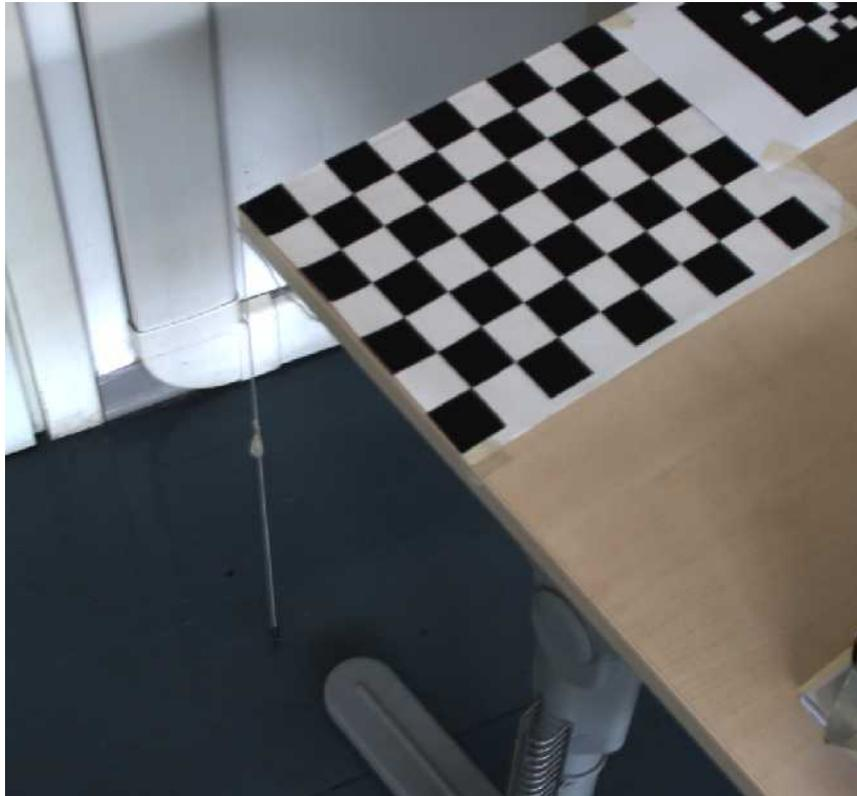
*The chessboard used to check the calibration of the camera chain.*
