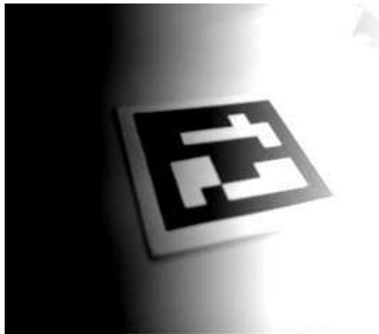
*Automatic thresholding allows ARToolKit Plus to work under several illumination conditions.*
