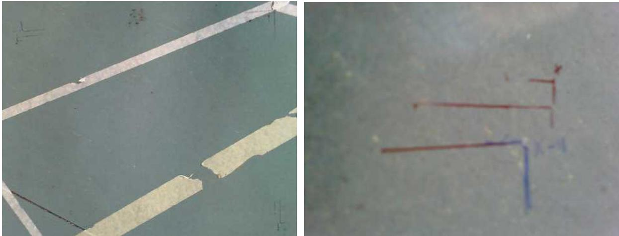
From top to bottom: drawing of the dima on the floor with a felt-tip pen in pose 18, measuring a movement of 1cm on x-axis and y-axis and one degree on theta, drawing of the new pose 18', close to the previous one.
