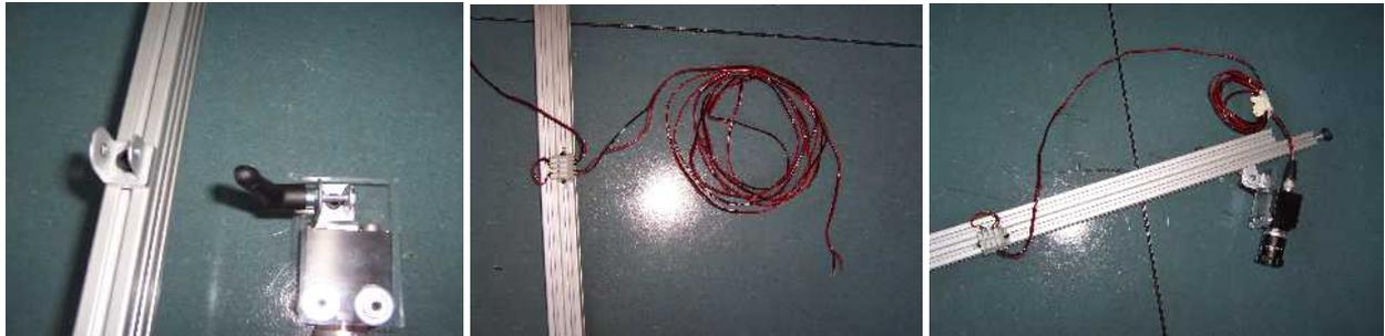
*Connecting the power of one of the four cameras and fixing the camera on a pole.*
