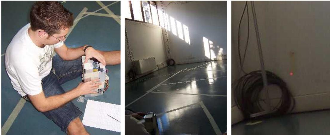
*(Left and centre) Taking distance measurements from the 3 robot-frame points to the world-points, with the hand-laser. (Right) Zoom of the central picture, to show the hand-laser spot and the world-point n. 5.*
