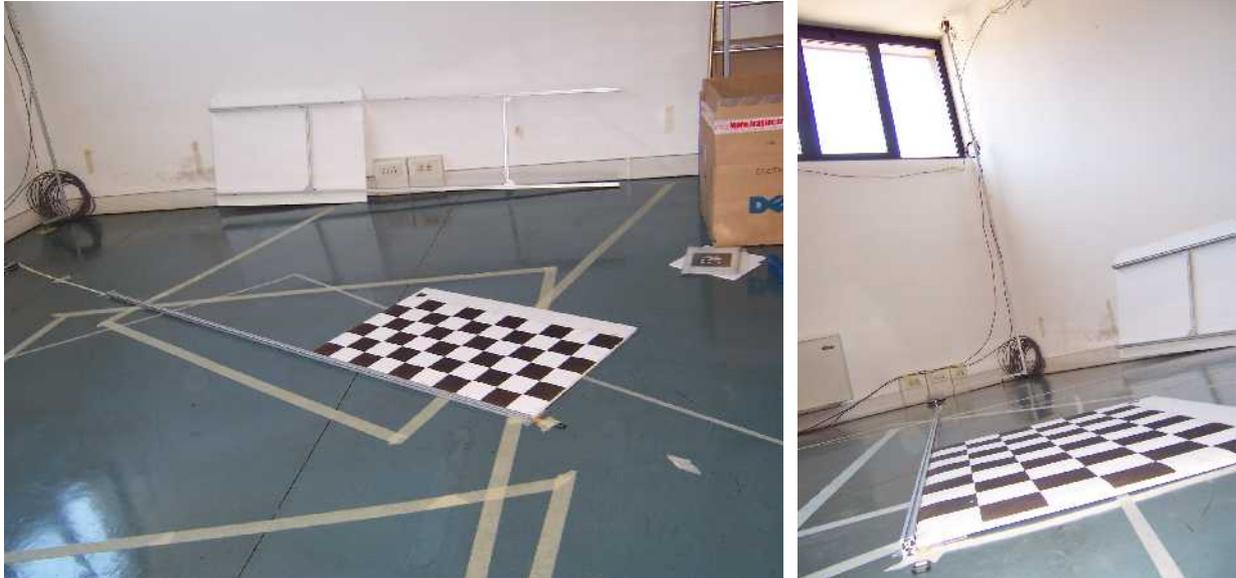
*Calibration pattern put in a known position with respect to the GTVframe, so to compute the camera-to-GTVframe roto-translation.*
