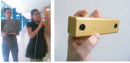
Fig. 1. Stereo vision system used to acquire the image sequences. (Left) Experimental setup during the data acquisition for the indoor experiment.
