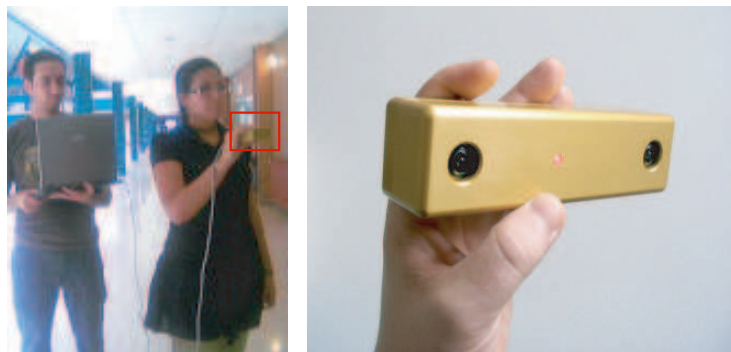
Figure 11: Stereo vision system used to acquire the image sequences. Picture on the left shows the experimental setup during the data acquisition for the indoor experiment.
