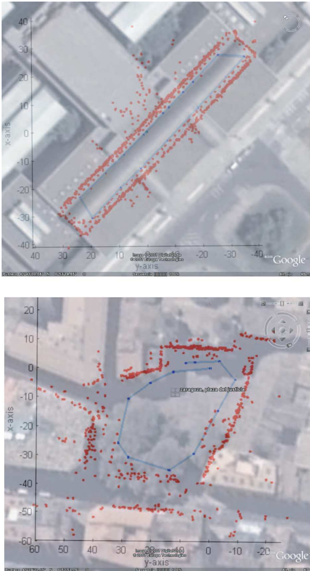
Fig. 9. Stereo visual SLAM recovers the true scale. (Top) Building environment and (bottom) the public square overlapping Google Earth.
