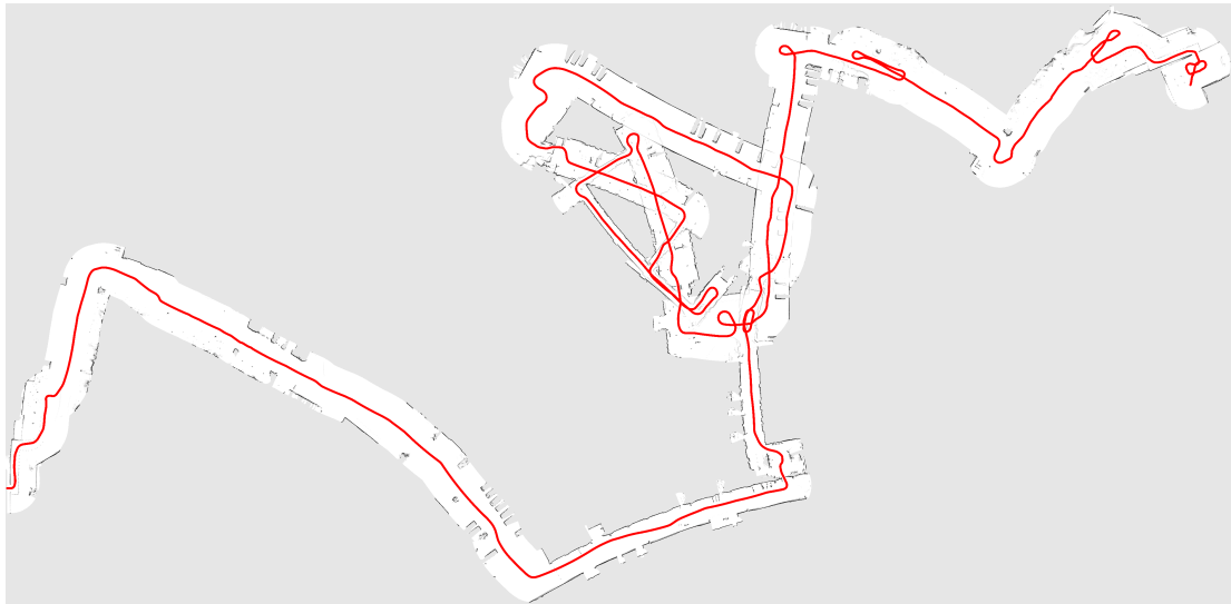
Outdoor/Bovisa 2008-10-04 Static: Maps generated from laser scans using improved odometry.
