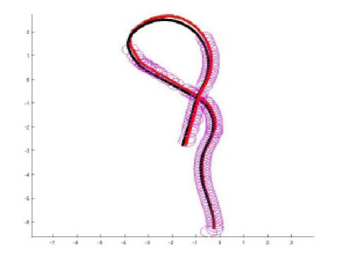
GT laser superimposed with GT vision. In black the odometry data stream.
