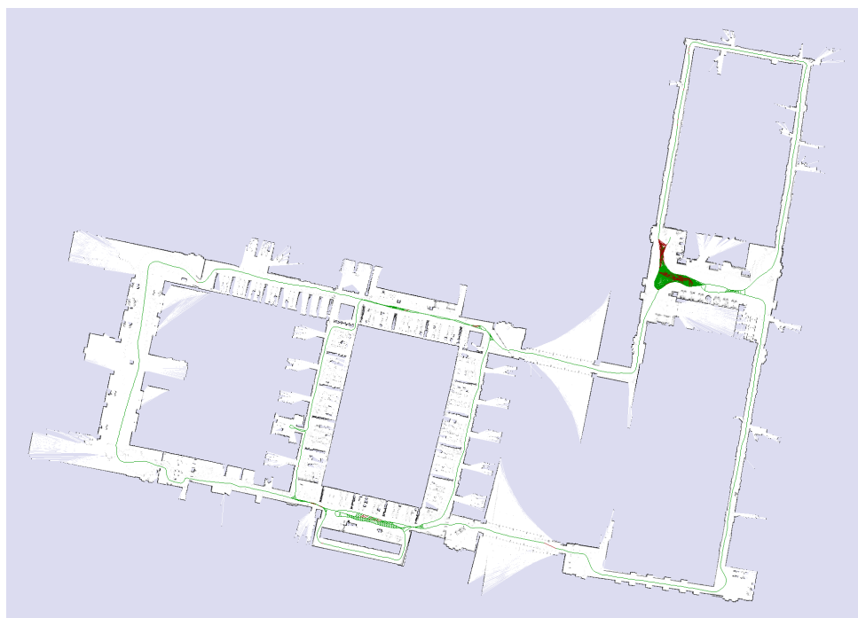
Figure 13: Result of GraphSLAM for the Bicocca 2009-02-26a dataset. Relations with an error over 0.2 m are colored red and below 0.2 m are colored green.
