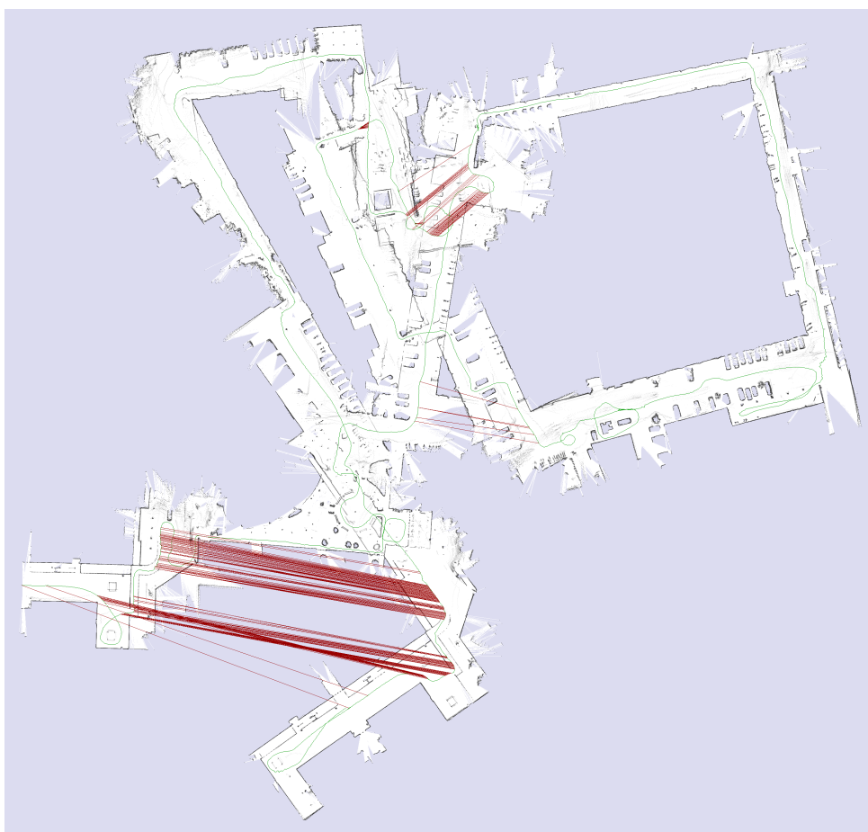
Figure 35: Result of the scan matching algorithm for the Bovisa 2008-10-07 dataset. Relations with an error over 1 m are colored red and errors below 1 m are colored green.
