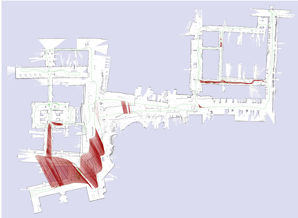
Figure 31: Result of the scan matching algorithm for the Bovisa 2018-10-06 dataset. Relations with an error over 1 m are colored red and errors below 1 m are colored green.
