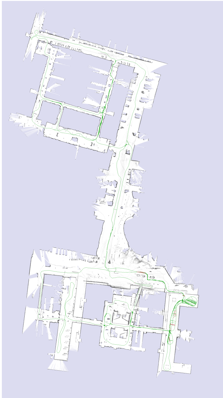
Figure 33: Result of GraphSLAM for the Bovisa 2008-10-06 dataset. Relations with an error over 1 m are colored red and errors below 1 m are colored green.
