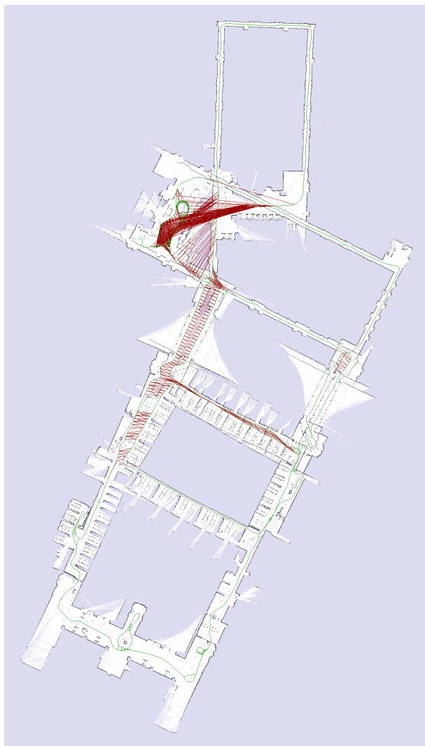
Figure 16: Result of RBPF for the Bicocca 2009-02-26b dataset. Relations with an error over 0.2 m are colored red and below 0.2 m are colored green.
