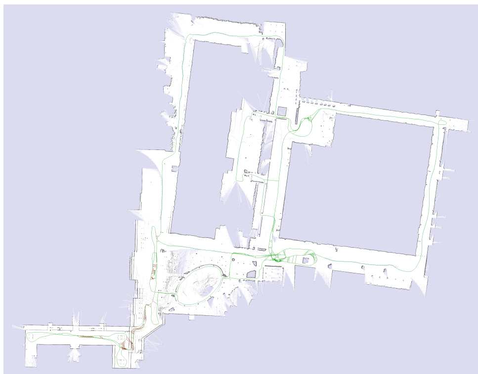
Figure 28: Result of RBPF for the Bovisa 2008-10-04 dataset. Relations with an error over 1 m are colored red and errors below 1 m are colored green.
