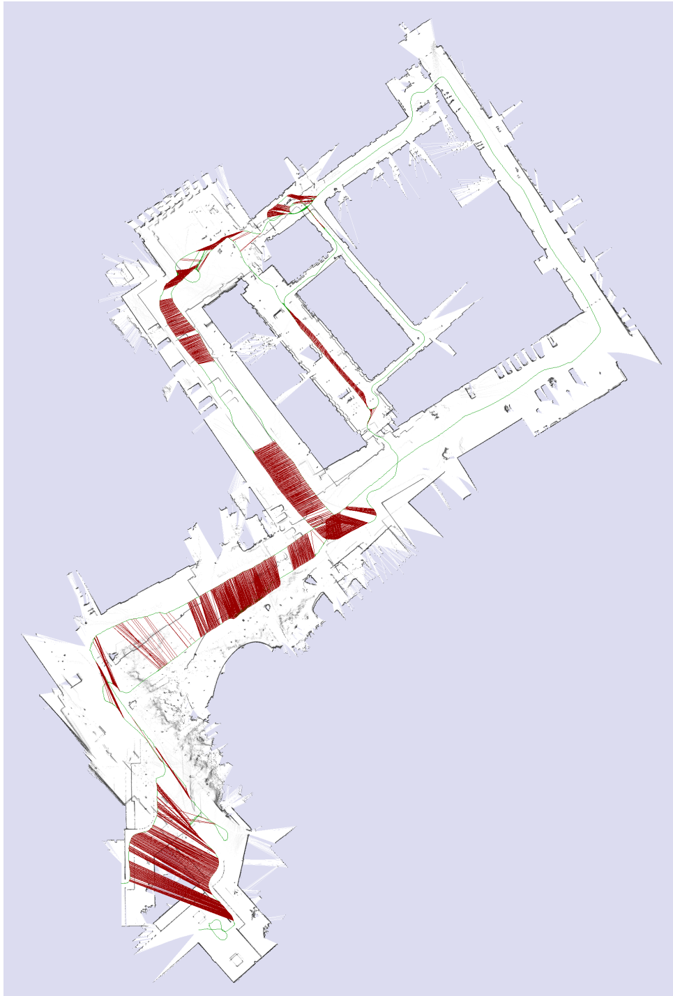
Figure 23: Result of the scan matching algorithm for the Bovisa 2008-09-01 dataset. Relations with an error over 1 m are colored red and errors below 1 m are colored green. The shown map has major inconsistencies and has also topological errors.
