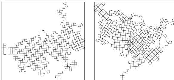
Fig. 7. The result of MLR strongly depends on the initial configuration of the network. (Left) Small initial pose error. (Right) Large initial pose error.
